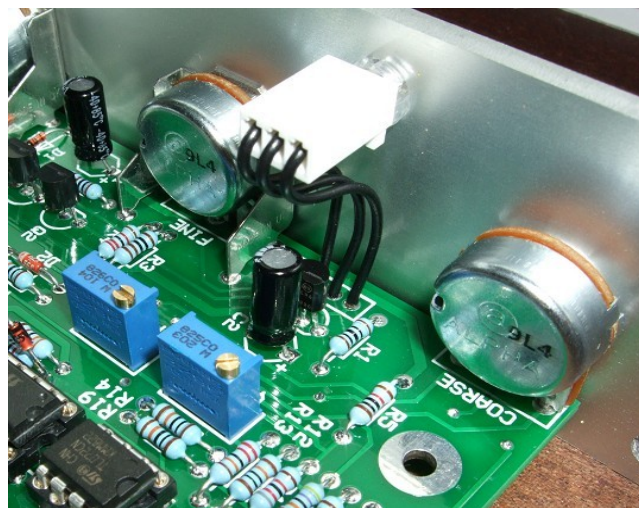
The three leaved tri-colour LED used in the VC-LFO module
