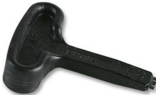
The special MTA hand tool needed to push the wire into the 0.1" IDC housings. Sadly a different tool is required for the 0.156" connectors.
