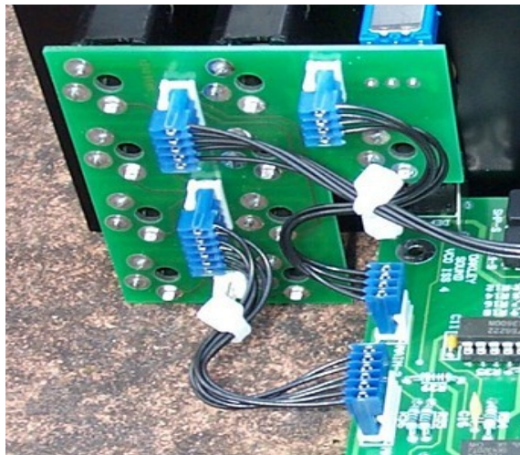
An example of MTA solderless interconnects on an older issue 4 VCO module. The dust covers have been left off to show the IDC termination within the blue housings. Cable ties hold each wire bundle in place and keep it neat.
