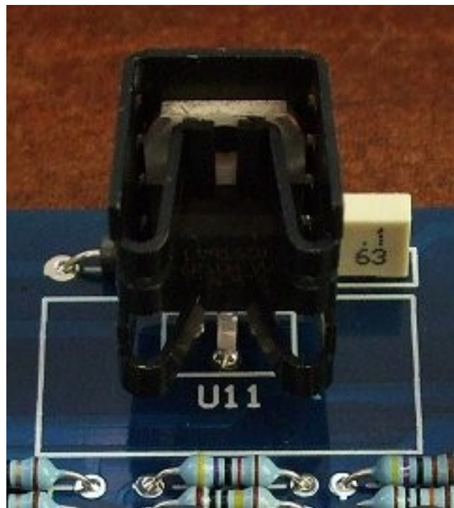
TO-220 power device in a small clip on heatsink on the Filtrex-II board. Note the middle leg of the device has been bent forward to fit into the board.
