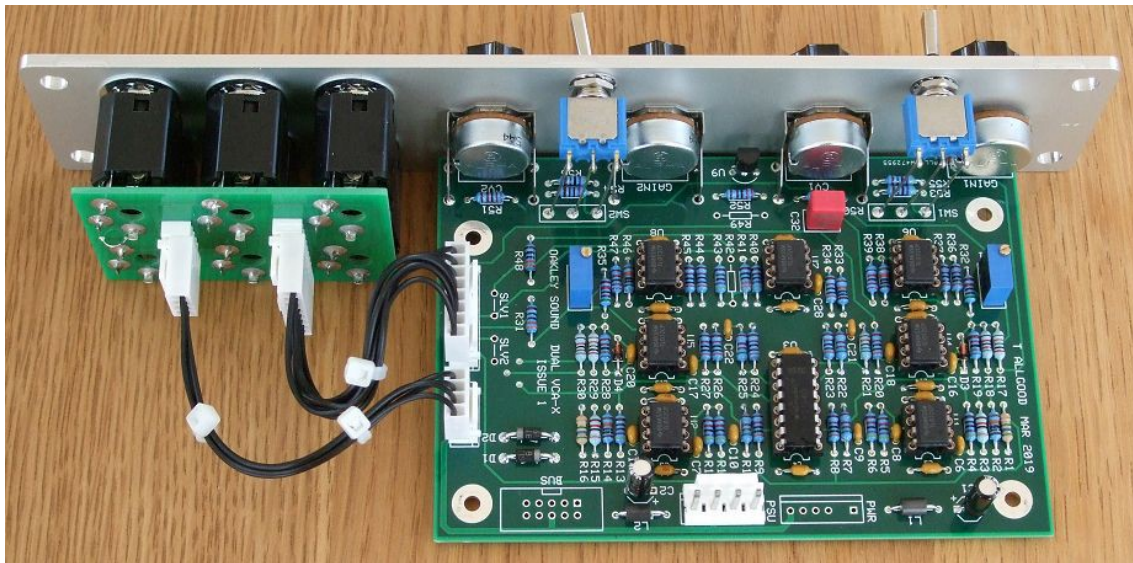
An Oakley Dual VCA-X module behind a natural finish 1U wide Schaeffer panel. Note the use of the optional Sock6 socket board to facilitate the wiring up of the six sockets.
