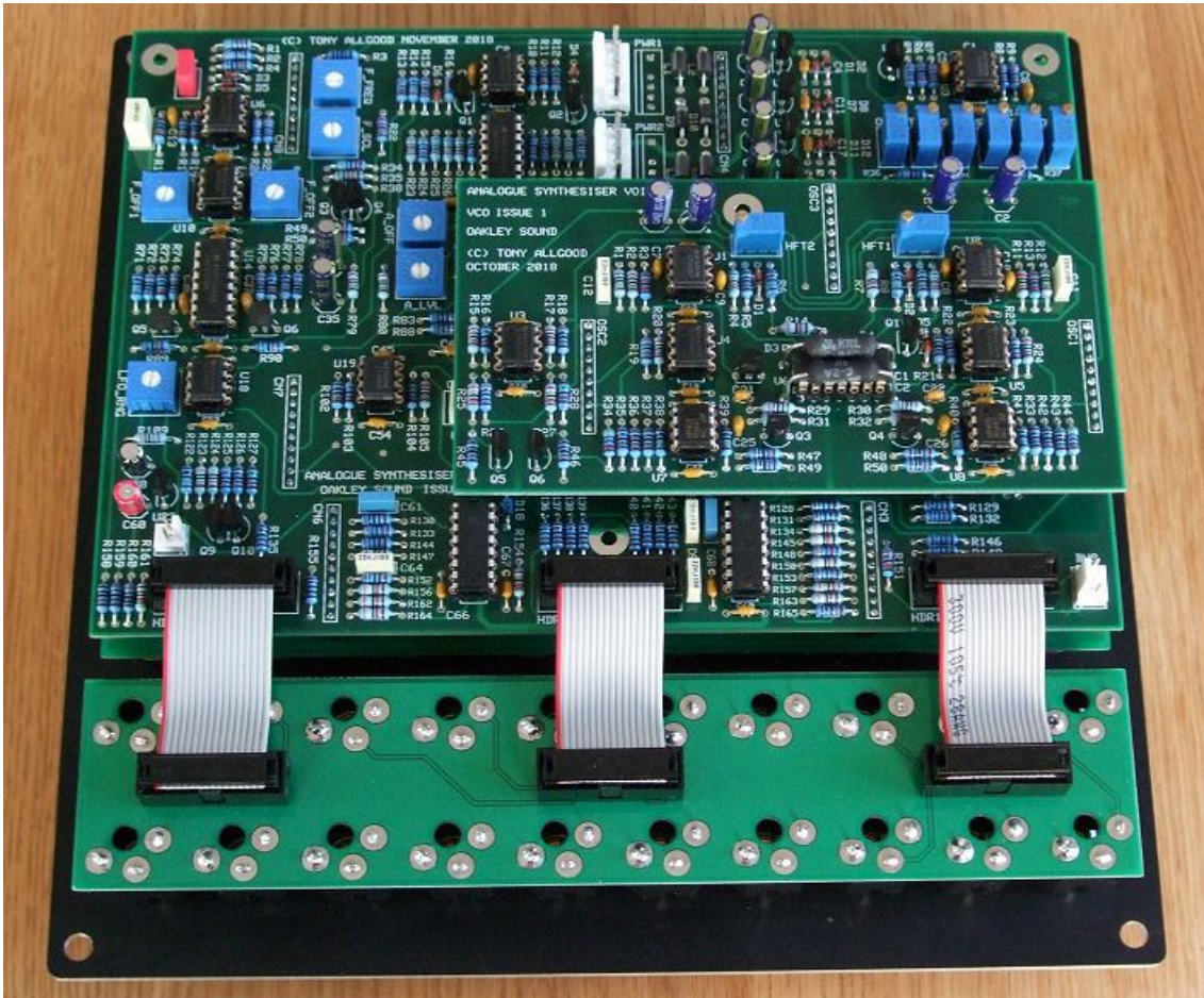
The prototype issue 1 ASV fitted to a MOTM format panel.
