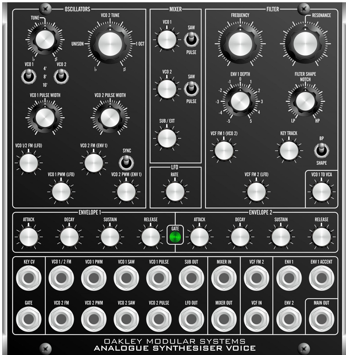
The 4MU wide panel design for the MU format module.
