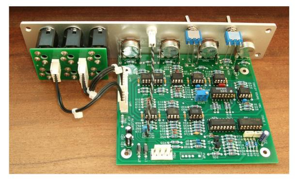
This is the prototype issue 1 VRG module behind a natural finish 1U wide MOTM format Schaeffer panel. Issue 2 modules are almost identical but feature the Oakley Bus CV and gate connection on the main board.
