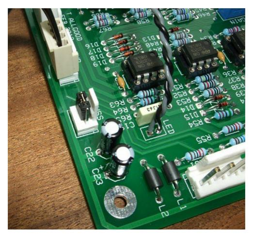
The three way BUSS header with jumper fitted. The jumper should be fitted if you are not using the Oakley Buss interconnections.
