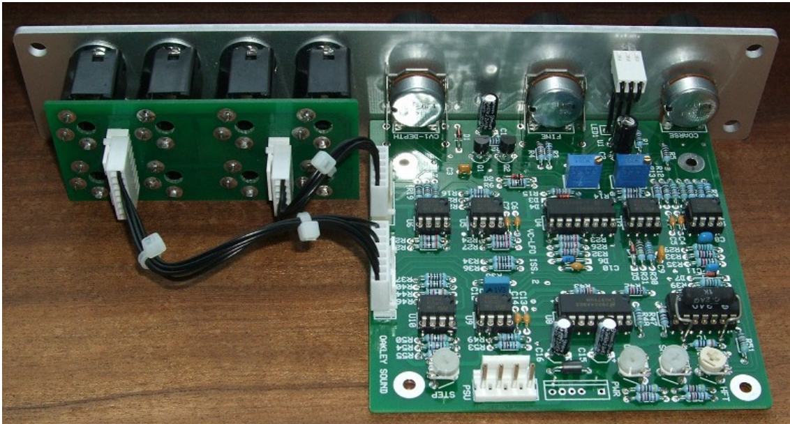
The issue 3 PCB mounted behind a natural finish panel. Note the use of the optional Sock8 socket board to facilitate the wiring up of all those sockets.
