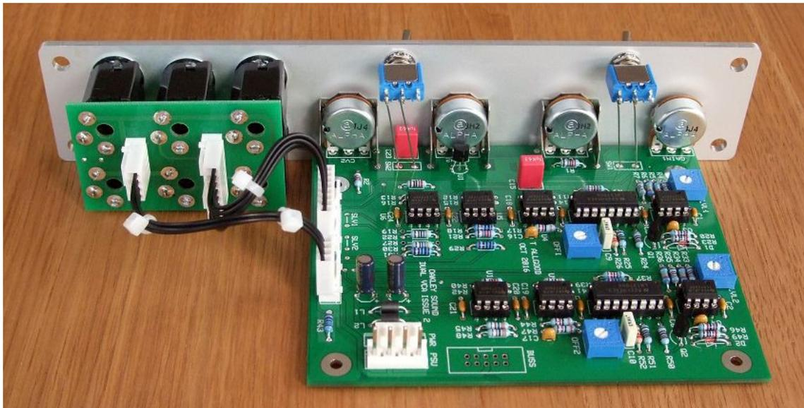
*This is the issue 2 Oakley Dual VCA module behind a natural finish 1U wide Schaeffer panel. Note the use of the optional Sock6 socket board to facilitate the wiring up of the six sockets.*
