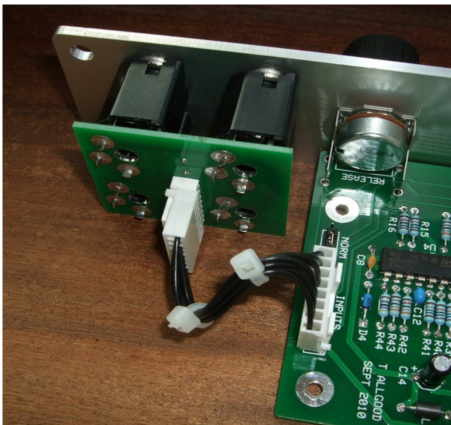
The Sock4 makes a very neat job of wiring up the four sockets.
