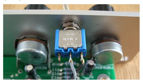
If you are fitting the switch then you need to connect it to the pad marked as SW1 on the Diode Superladder PCB. The switch is wired with a twisted wire pair. This is made by twisting two pieces of insulated multistrand wire together tightly to form a simple cable. You can use two different colours but you don't have to as it does not matter which wire connects to which lug on the switch. Here I have used black and grey wires.
