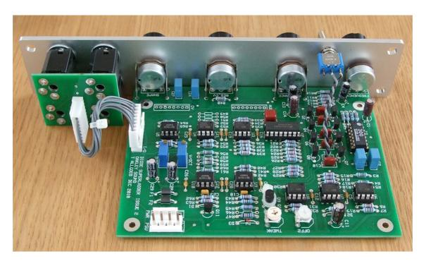
This is the older issue 2 Oakley Diode Superladder module behind a natural finish 1U wide Schaeffer panel. Note the use of the optional Sock4 socket board to facilitate the wiring up of the four sockets.
