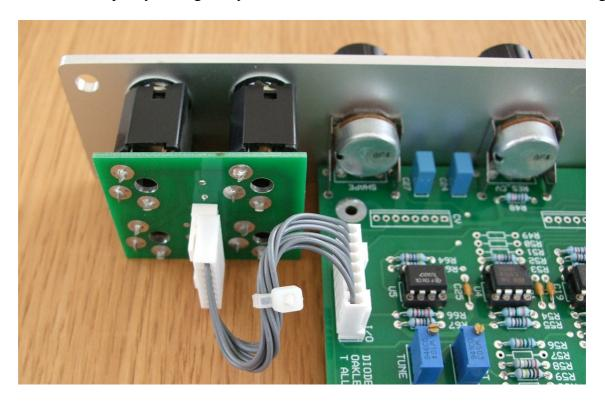
The prototype Diode Superladder filter core module showing the detail of the board to board interconnect. Here I have used the Molex KK 0.1" system to connect the Sock4 to the main PCB.
