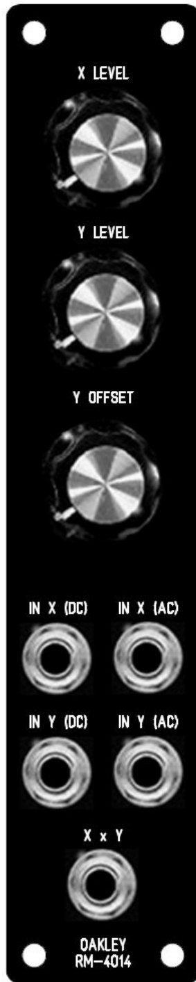
The suggested 5U panel design. Note the slightly different spacing of the knobs compared with the usual 41mm 5U Oakley standard.
