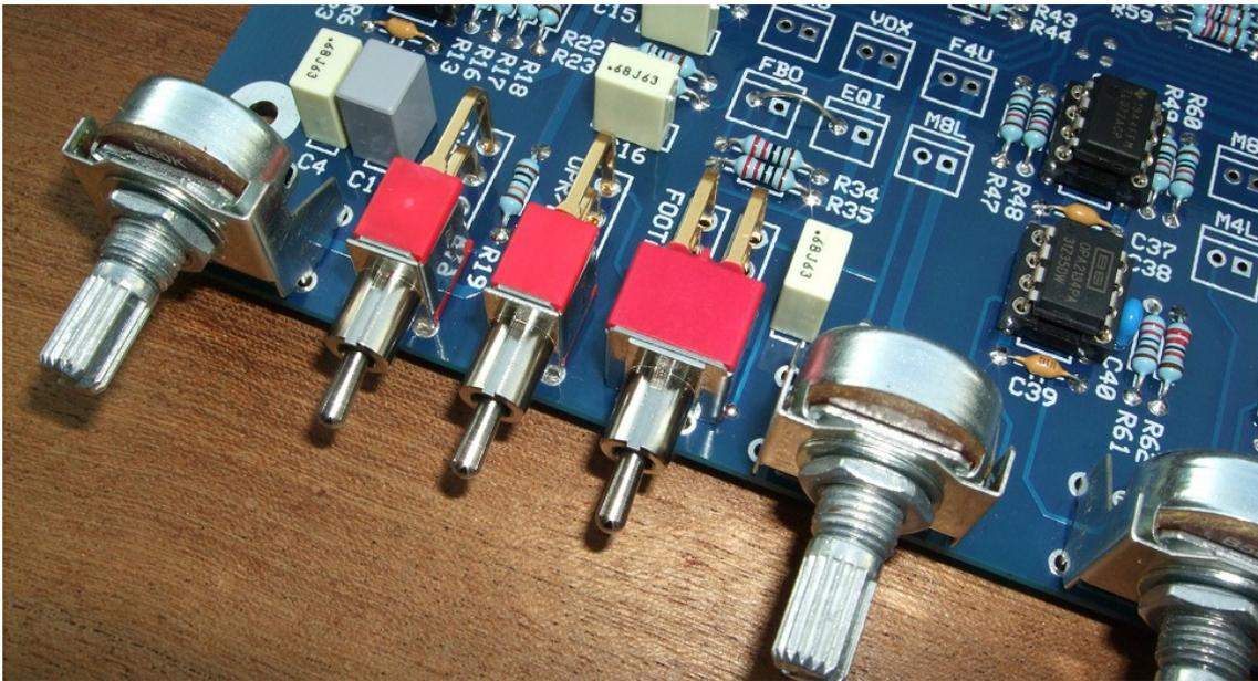
*The three switches. These are made by Multicomp (part numbers 1MS1T2B4M7RE for the two SPDT and 1MD1T2B4M7RE for the single DPDT.)*
