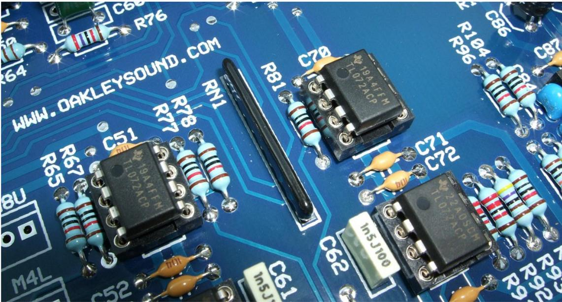
*A close up of the resistor network. This is eight resistors in one package manufactured so that one end of all the resistors are tied to one pin – usually labelled with dot or a line.*
