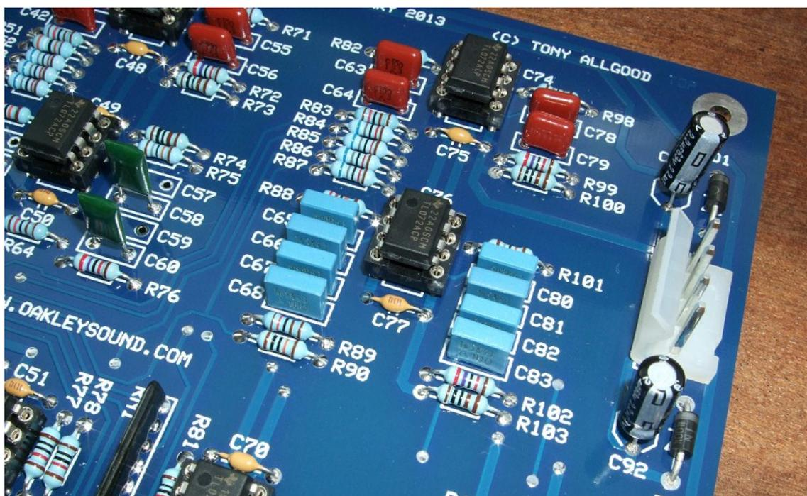
*The power header on the HVM board. This is a 0.156" (3.96mm) Molex KK. This is similar to the MTA156 type connector that we normally use on our MOTM compatible modules but the two are not interchangeable. However, the KK is cheaper and only requires a cheap crimper to make the leads.*
