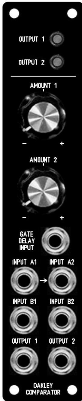
The suggested 1U wide panel layout for the issue 2 Dual Comparator and gate delay module.
