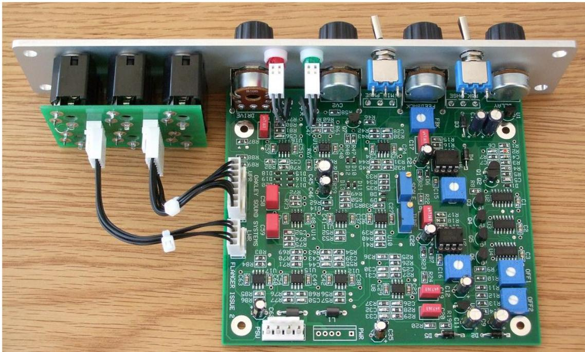
*The issue 2 Oakley Flanger as a single width MOTM format module in a natural finish Schaeffer panel. Note also the use of the optional Sock6 socket board to help keep the wiring to the sockets neat and tidy.*
