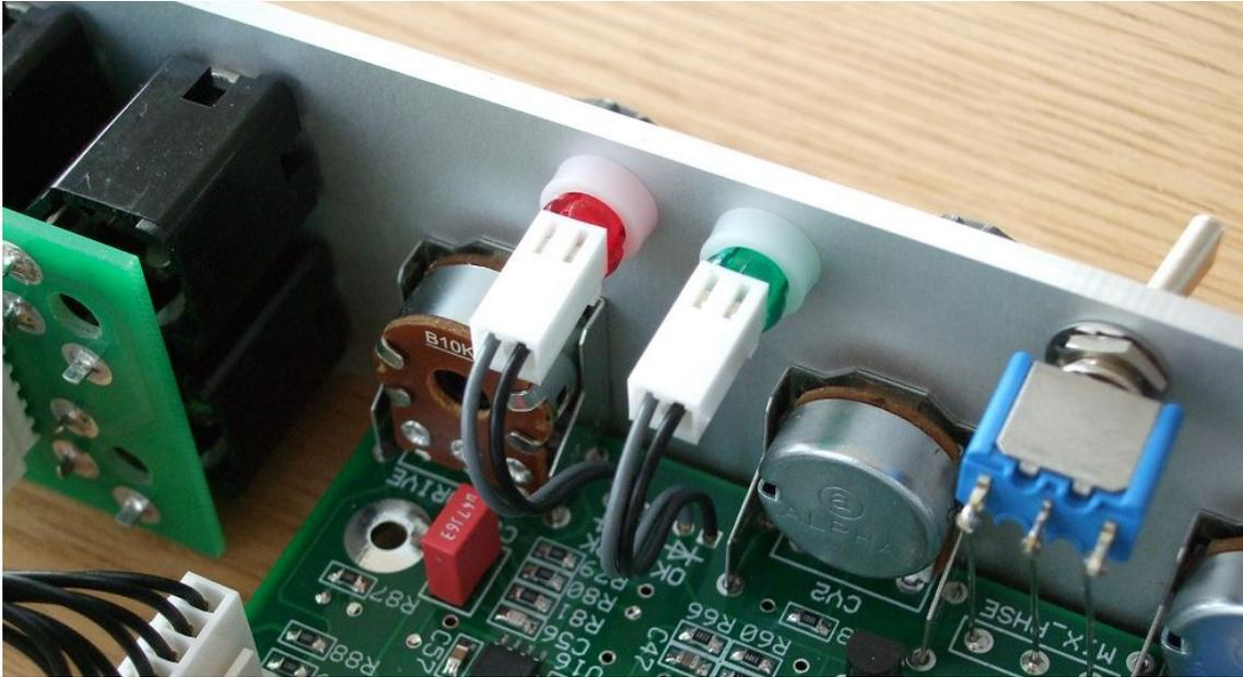
*Here I have used a Molex 0.1" KK header and crimps to attach each LED to the PCB. The LED is thus not soldered to the wiring allowing the board to be easily removed from the front panel.*
