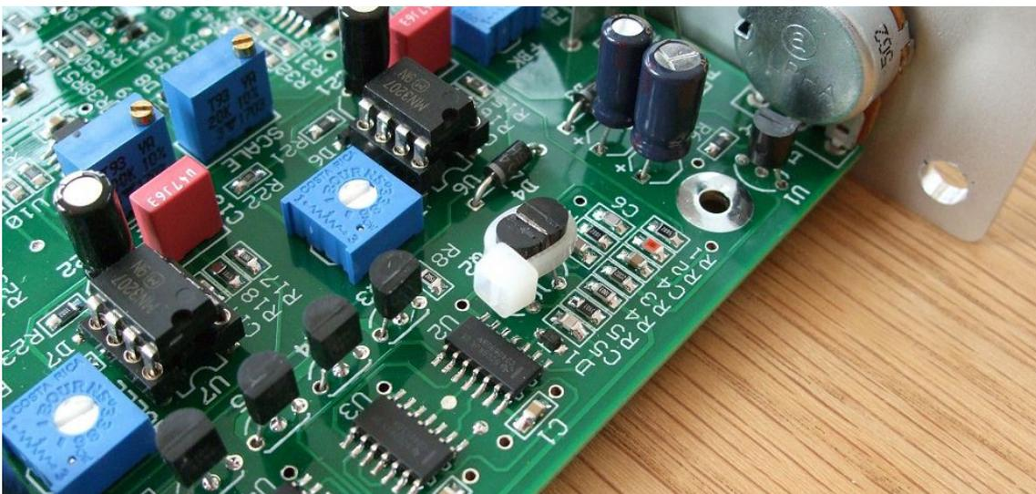
*Q1 and Q2 can be secured together with a cable tie as shown to reduce the amount of clock frequency drift with temperature. A very thin layer of heat sink paste between them improves the thermal bonding.*
