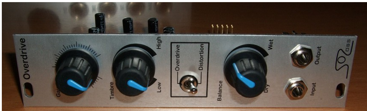
The Oakley Overdrive module for the Eurorack format. This module has been built by Krisp1.
