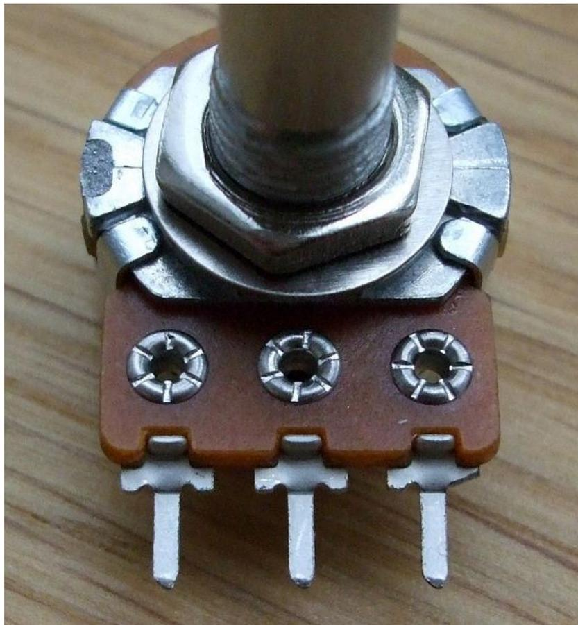
As can be seen in the above photograph above all we need to do is snip off a portion of the right hand locating lug on the right most pin. You can see that the right pin has been modified when compared to the other two pins and that a diagonal cut has been made removing some of the pin's metal.
