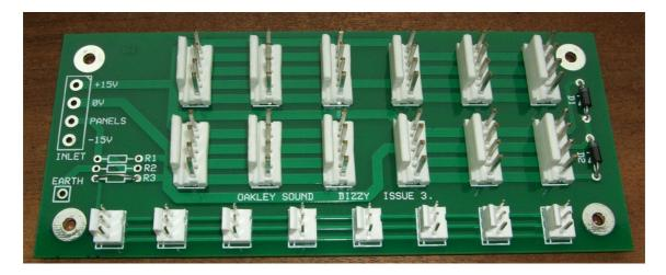
The issue 3 Dizzy board fitted with MTA156 power headers and Molex KK 0.1" headers for the Oakley Bus. The four way power inlet has not been fitted since this particular board will be hard wired to an Oakley PSU.
