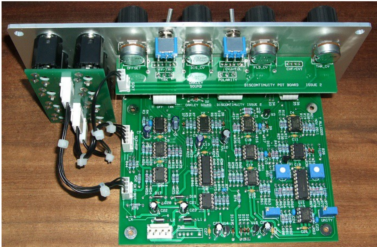
The prototype issue 2 module behind a natural finish Schaeffer panel in the MOTM format.
