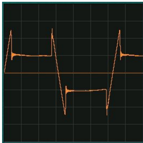
Figure 5. Discontinuity on both negative and positive parts of the input waveform. Discontinuity is set at around 40% of the threshold voltage.
