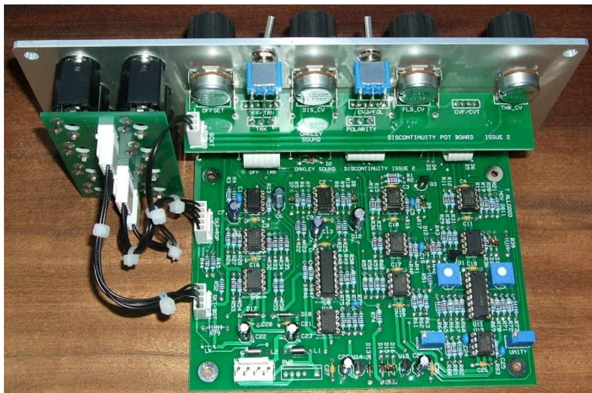
The prototype issue 2 module behind a natural finish Scheaffer panel in the MOTM format.
