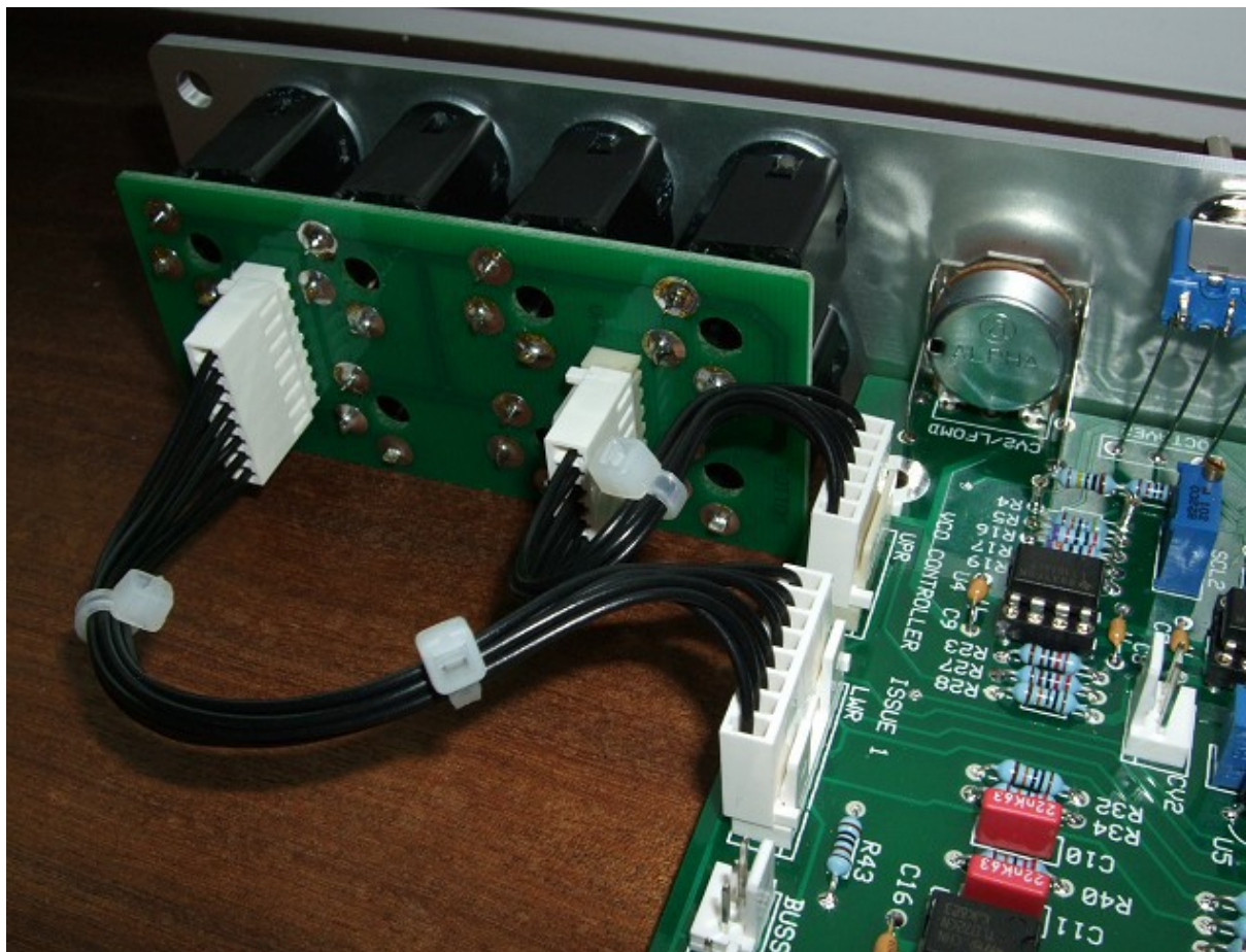
The prototype unit showing the detail of the board to board interconnects. Here I have used the Molex KK 0.1" system.
