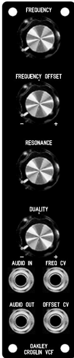
The suggested panel layout for the single width MOTM format module.
