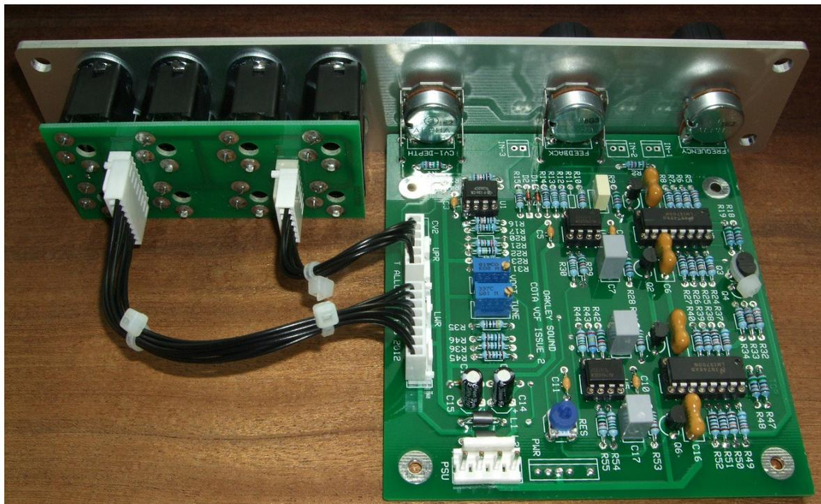
*The issue 2 prototype COTA in a 1U MOTM format panel with Schaeffer's natural finish. Note the use of the Sock8 socket board to make wiring so much easier and quicker.*
