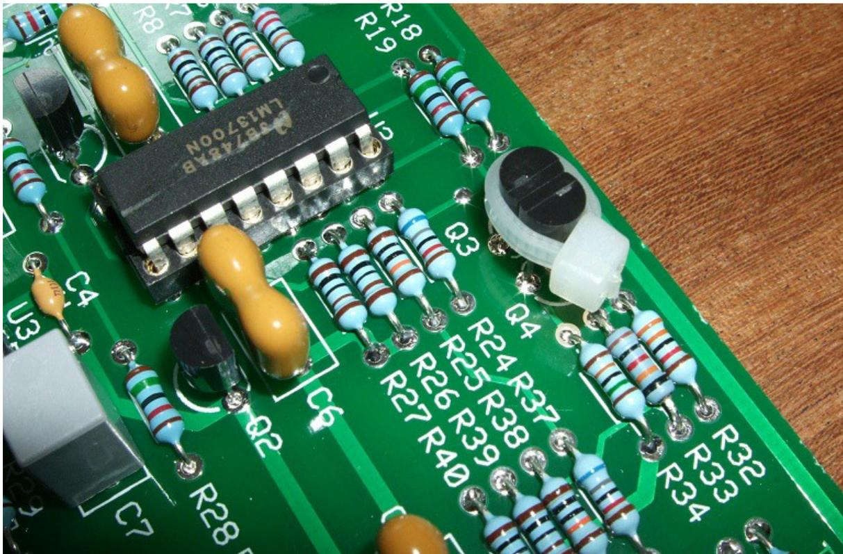
*Close up of the board showing the two bipolar transistors coupled together with a cable tie. You could use some thermal paste between them. This would thermally couple the two devices even closer but it is probably not worth it for this application.*
