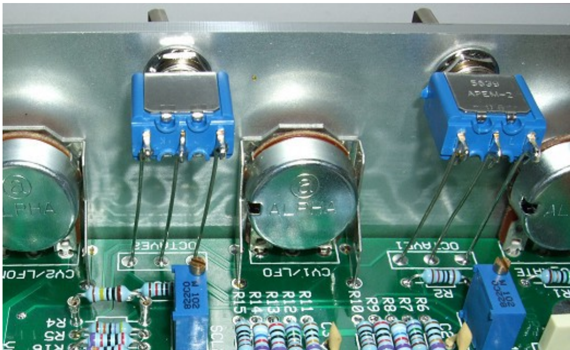
This is the VCO Controller module and shows the two panel switches connected to the PCB by solid core wire. Note the little hooks that wrap around the switch's connection tangs which keeps them in place while you solder.
