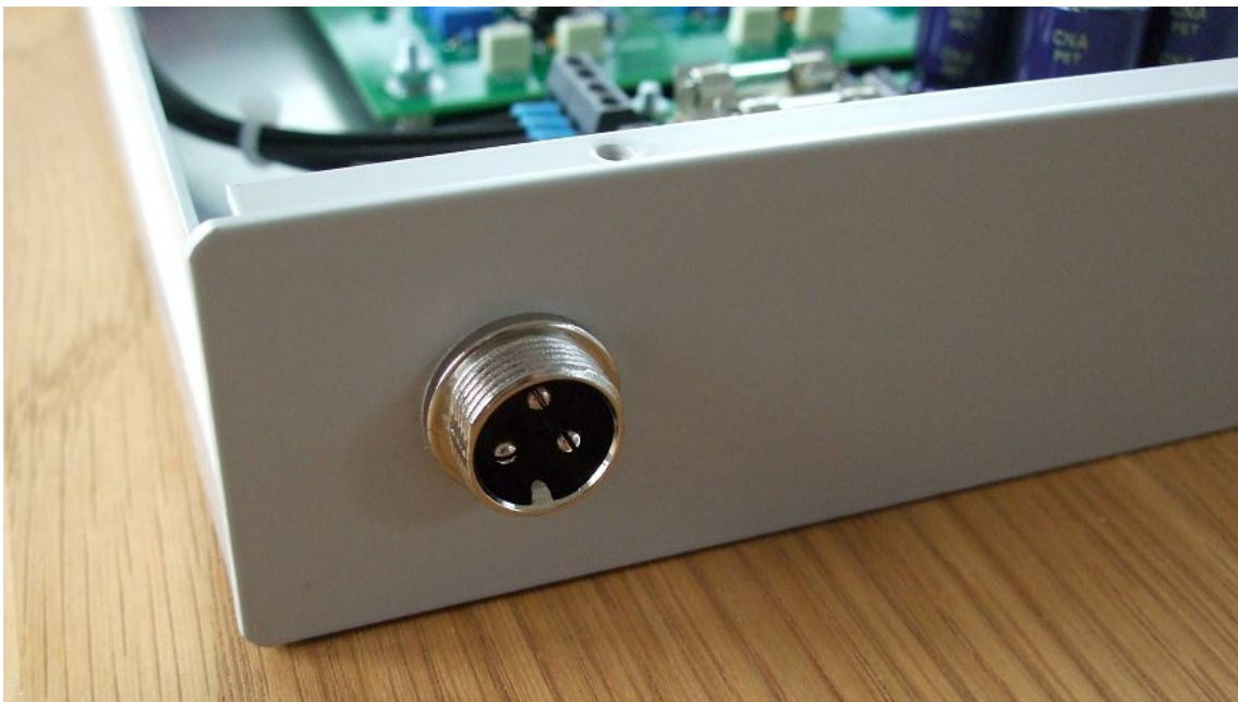
The three way power socket that will fit the Yamaha PA20 or PA30 power supply.
