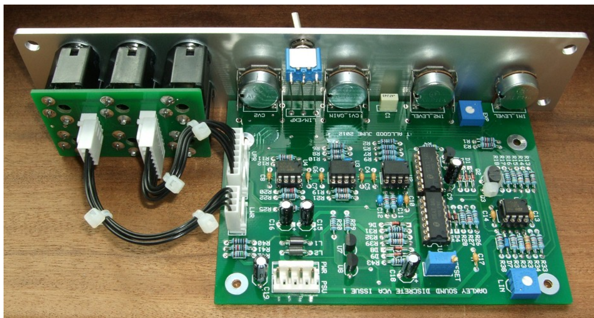
The issue 1 Oakley Classic VCA module behind a natural finish 1U wide Schaeffer panel.
